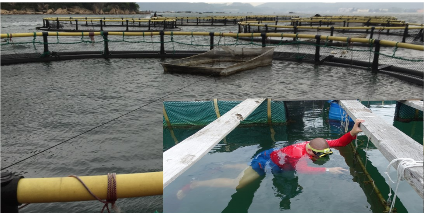
Dr. Wong examining copper-alloy netting being used in Shenzhen to reduce bio-fouling of aquaculture net pens, as part of collaborative research projects with Wieland Industries
